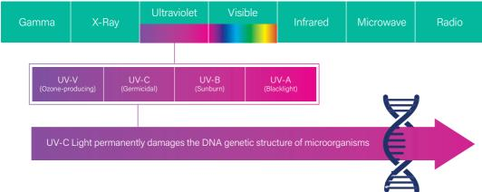
Ultra-V Connect<sup>™</sup> emits its UV-C rays via 3 single-ended, germicidal lamps. The constant UV output provided over their 9,000 hour life makes them a reliable and highly efficacious disinfection system.
