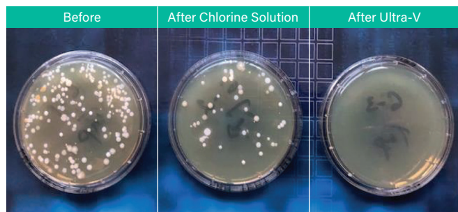
Figure 1: TVC on the sink in room 6
